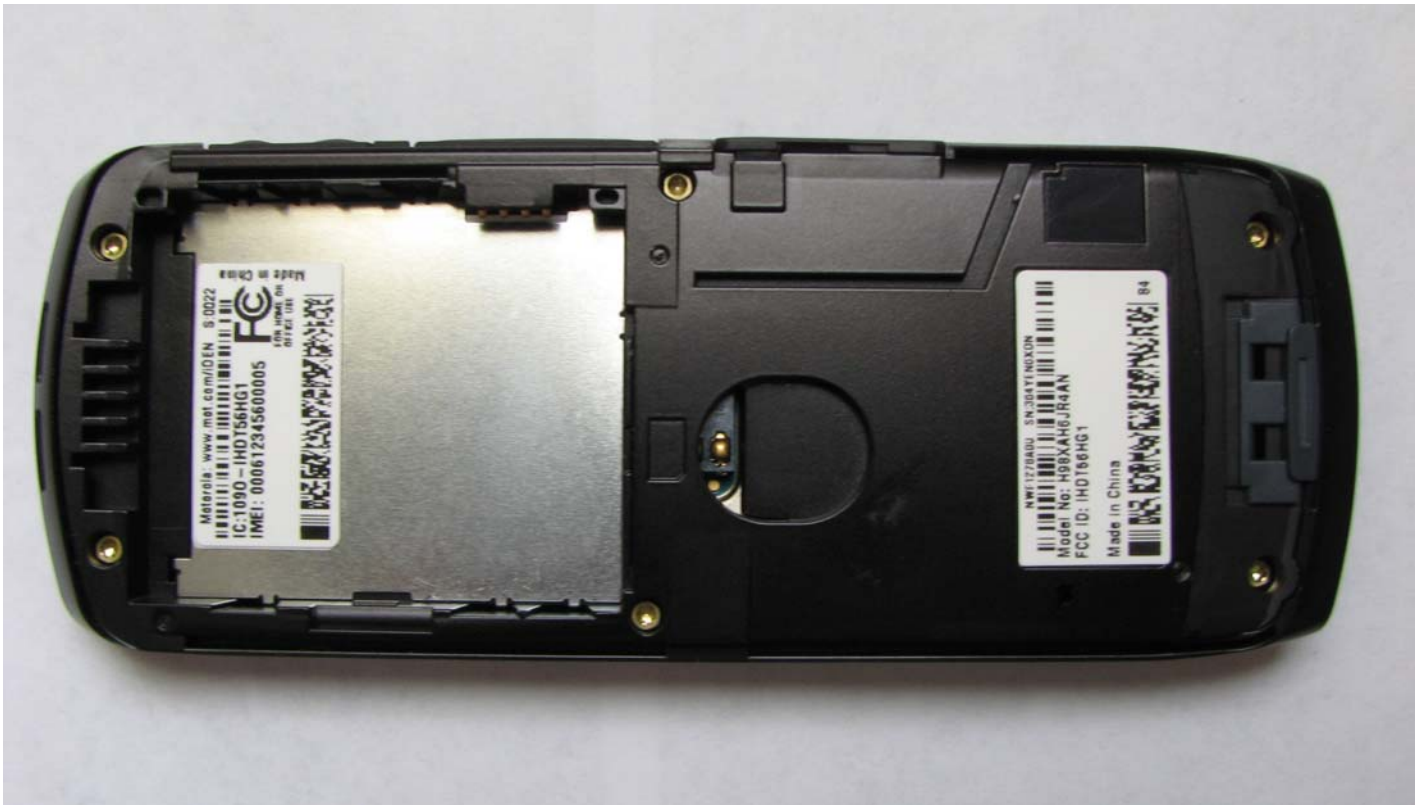
Figure 3-7. Battery Compartment of i290 radio.
