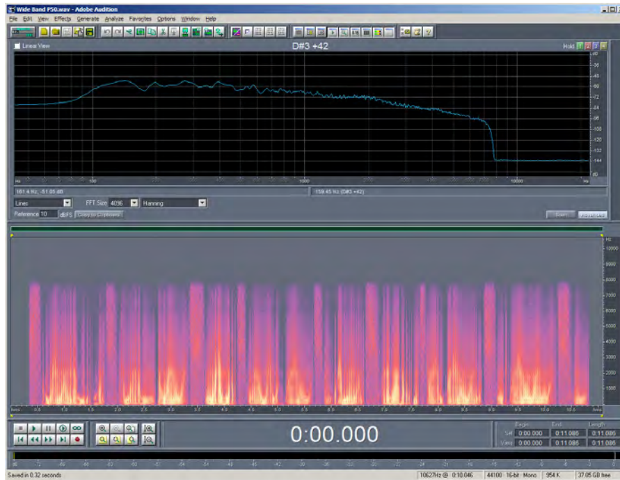
Figure 6.4.1-2 Wide Band P50 Frequency Response and Temporal Response Hanning Windowing Function and 4026 FFT Size
