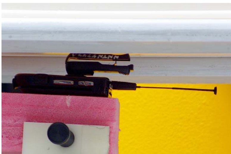
Figure 4: Body Assessment DUT w/Belt Clip against the phantom. (Same position used for antenna retracted)
