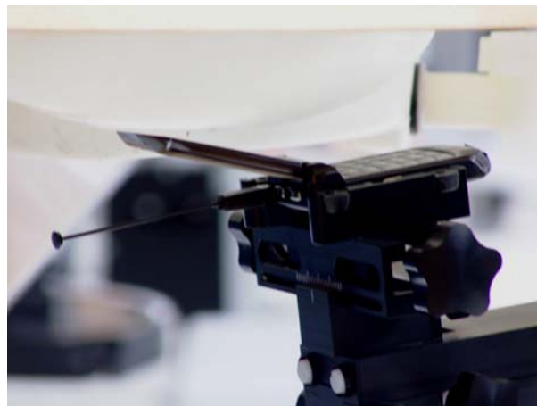
Figure 8: Assessment at the Head DUT at the Right Ear in Tilt position. (Same position used for antenna retracted)
