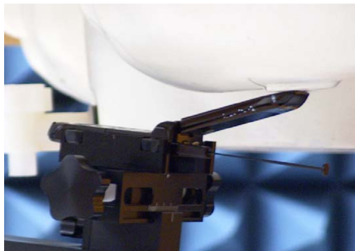
Figure 10: Assessment at the Head DUT at the Left Ear in Tilt position. (Same position used for antenna retracted)
