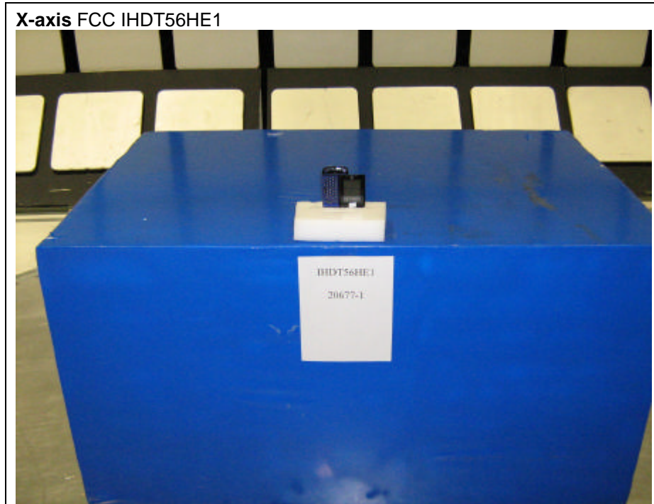
Figure 1 Test setup for Radiated Emissions
