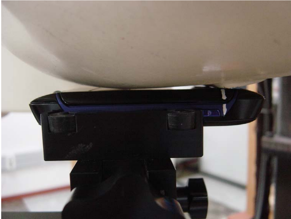
Figure 5: Phone Against the Head Phantom (Cheek Touch)
