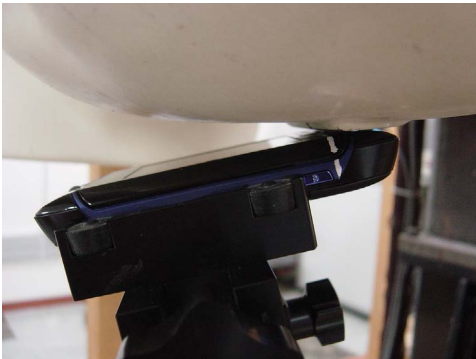
Figure 6: Phone Against the Head Phantom (15°Tilt)
