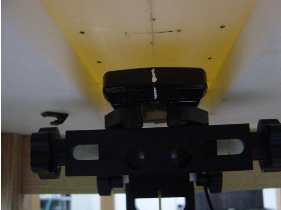
Figure 7: Phone Against the Flat Phantom (Sidekick slider closed)
