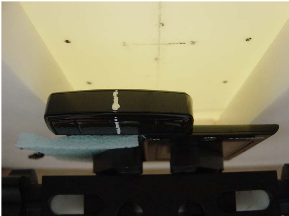
Figure 8: Phone Against the Flat Phantom (Sidekick slider opened)
