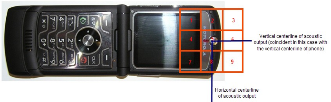
Figure A5-2. Phone Open - Orientation of Wireless Device and Measurement Plane
