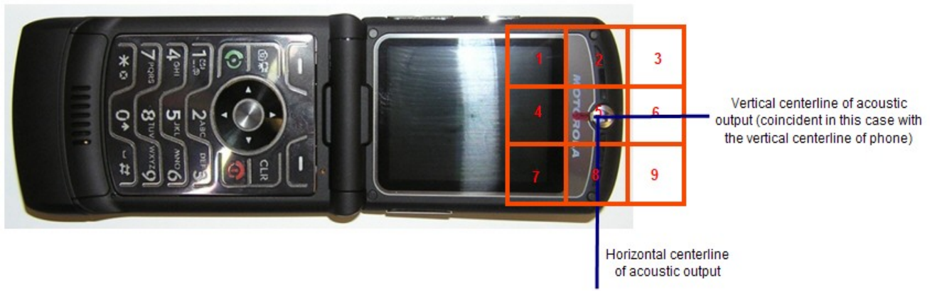
Figure A4-2. Phone Open – 5cm x 5cm grid for Near Field Measurements
