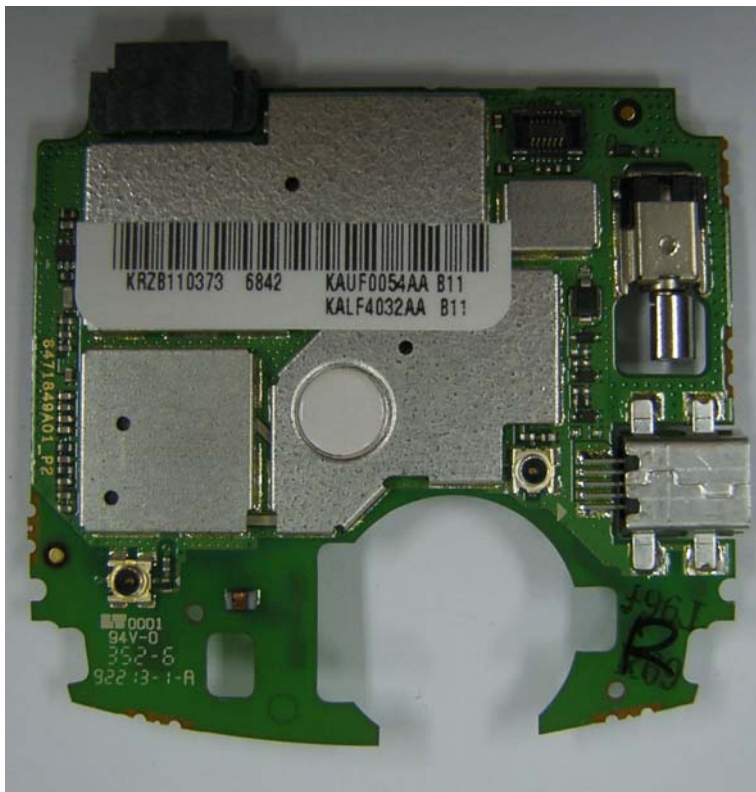
Main Board(shield on)
