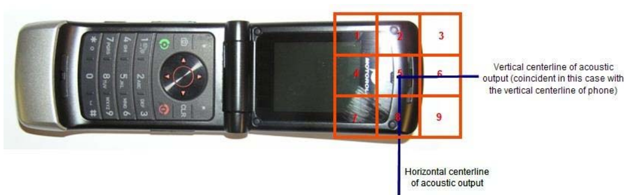
Figure A4-3. Phone Open – 5cm x 5cm grid for Near Field Measurements
