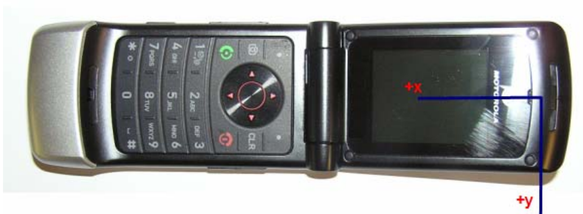
Figure A4-2. Phone Open – Coordinate Axis for T-coil Measurements
