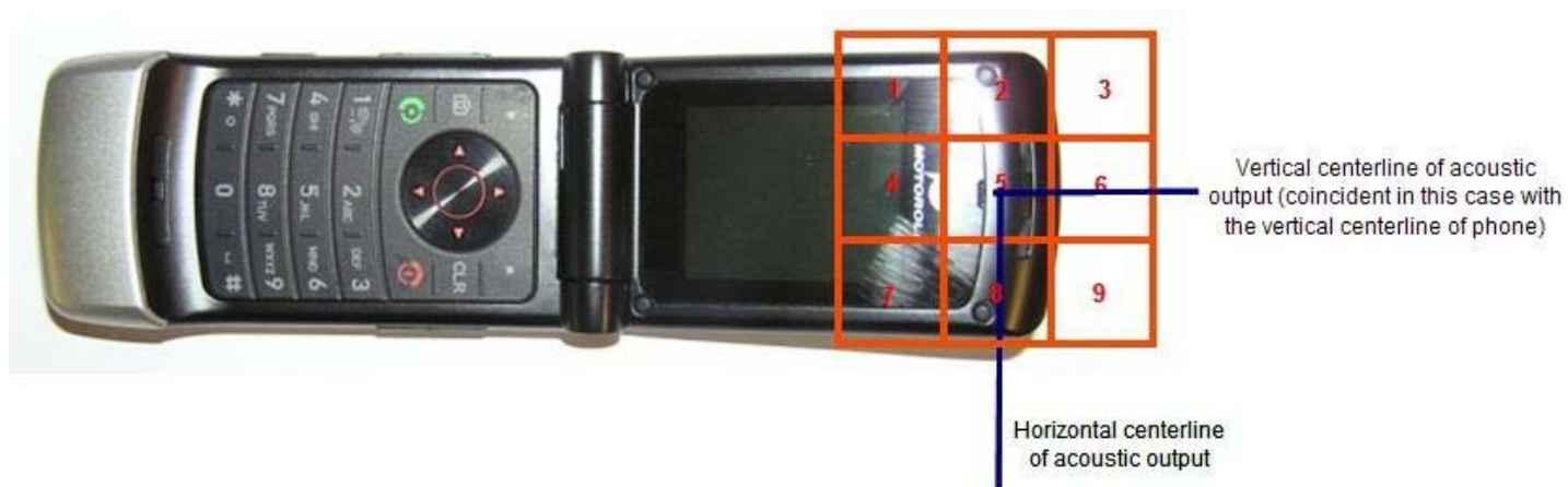
Figure A6-2. Phone Open - Orientation of Wireless Device and Measurement Plane
