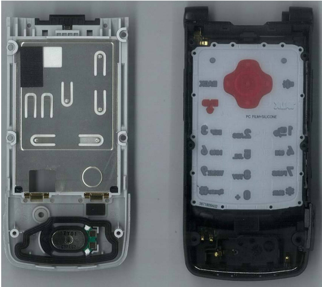
Inside Rear housing of Main Board
