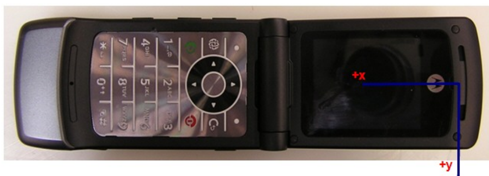
Figure A5-3. Phone Open – Coordinate Axis for T-coil Measurements
