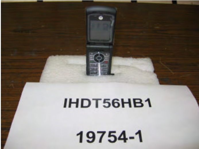
Radiated Emissions X-Axis
