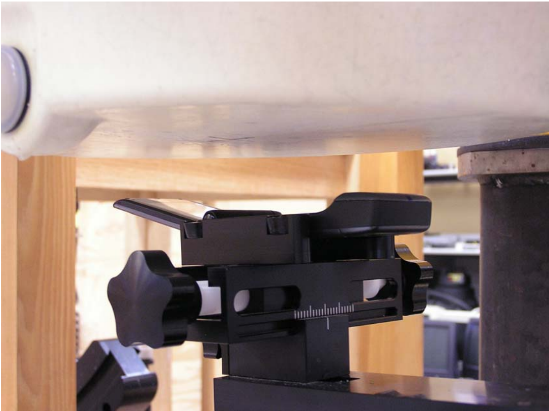
Figure 8 – Transceiver in Push-to-Talk position, Front of Phone 25 mm from Phantom position
