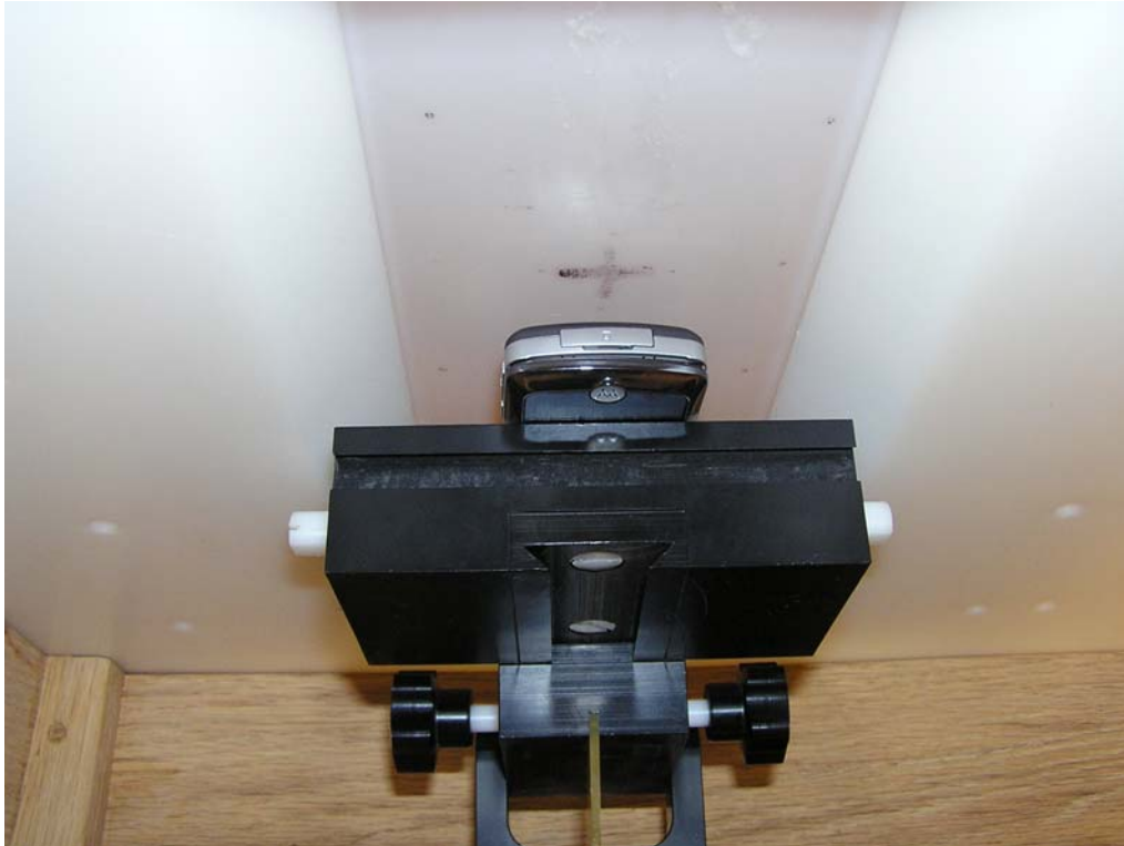
Figure 10: Bodyworn Back of Phone 15mm from phantom
