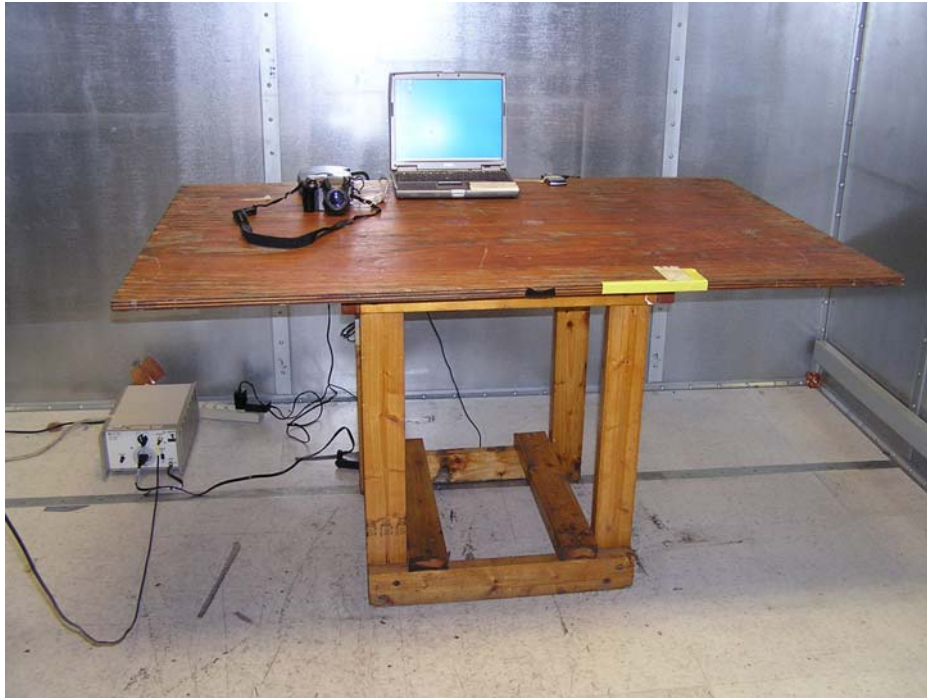
Figure 1. AC Line Conducted Emissions Measurement Setup
