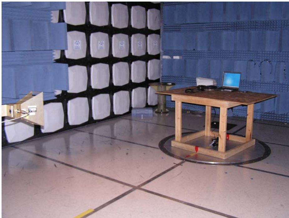
Figure 2. Part 15 Radiated Emissions Measurement Setup
