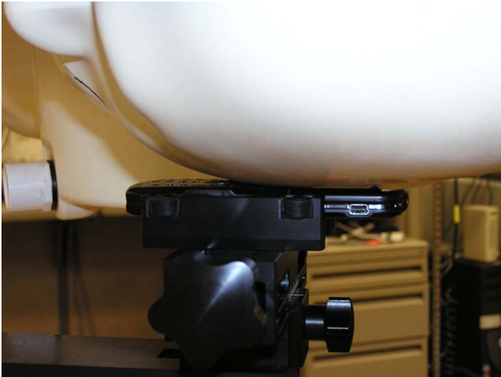
Figure 3. Phone Against the Head Phantom (Cheek Touch)
