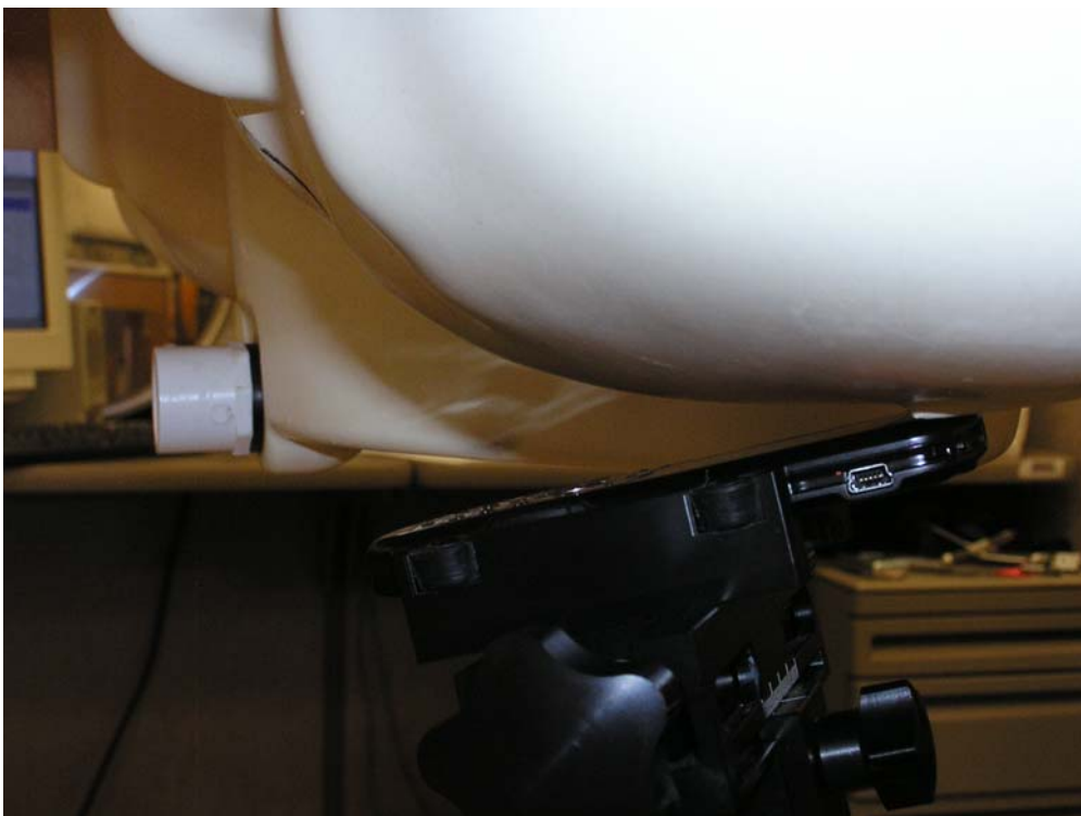
Figure 4. Phone Against the Head Phantom (15°Tilt)
