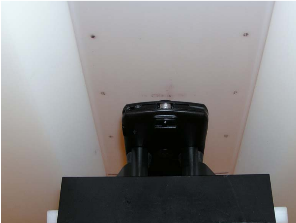
Figure 5. Phone Against the Flat Phantom
