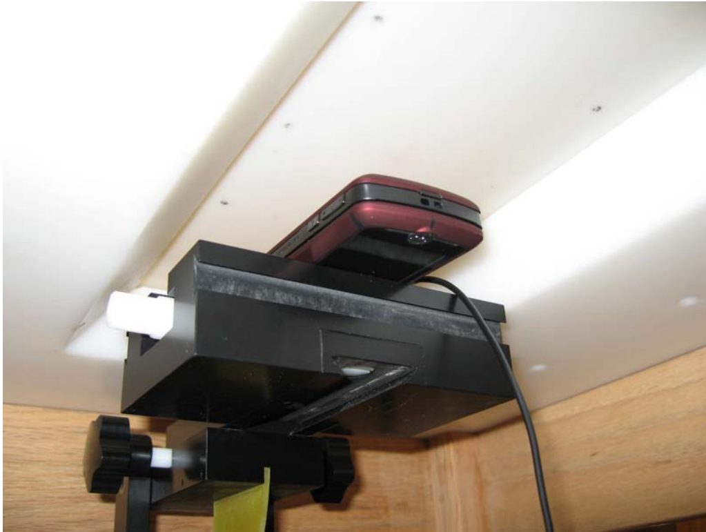
Figure 11 – Transceiver against body, Back of Phone 15mm from Phantom position
