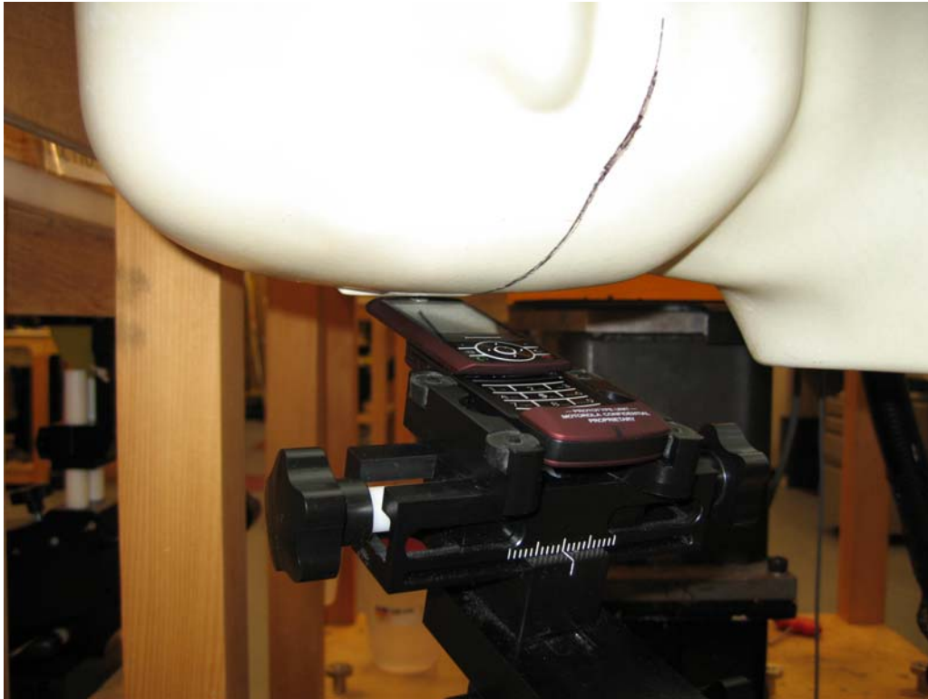
Figure 7 – Transceiver against head, 15° Tilt position, Slider Extended
