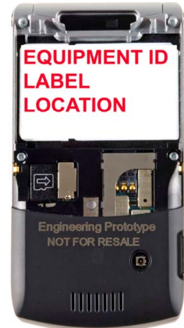
BACK OF PHONE WITH BATTERY COVER REMOVED
