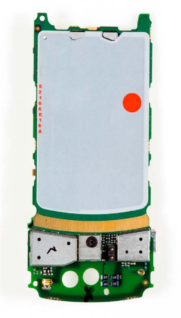
Main Board Top With Popples and Shields
