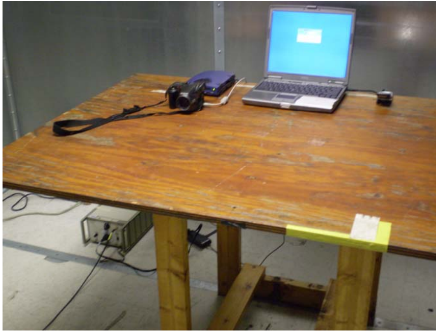
Figure 1. AC Line Conducted Emissions Measurement Setup
