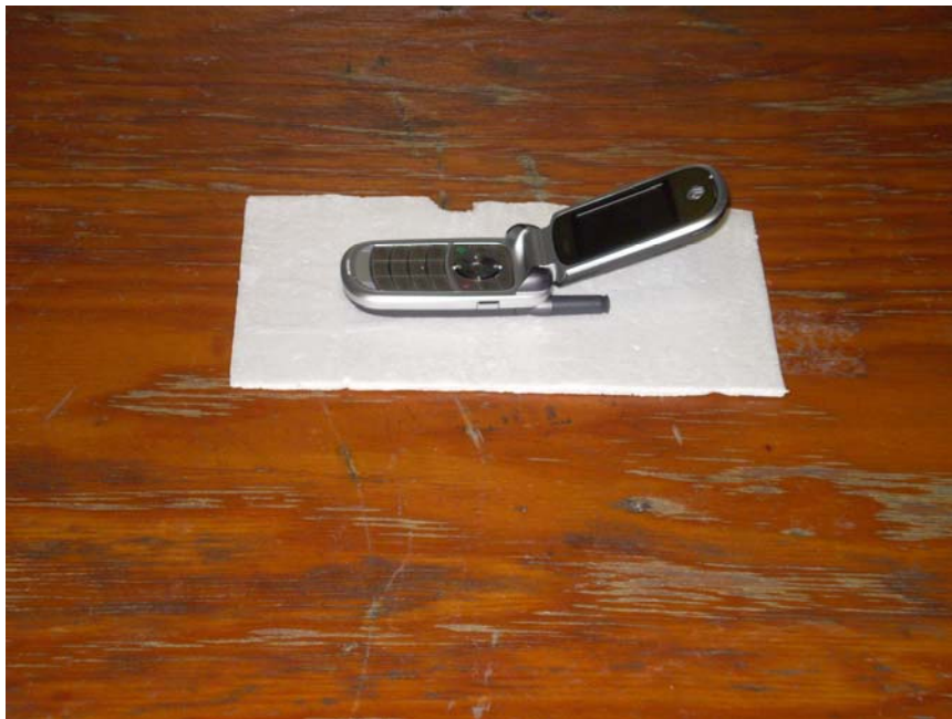
Figure 6. Radiated Emissions Z-Axis
