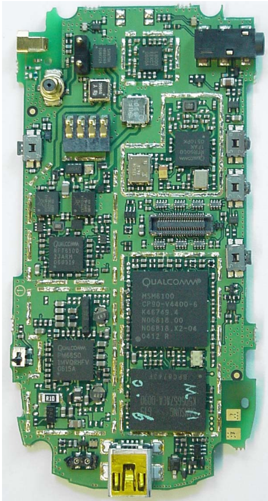
Figure 1: Board with Shields Removed
