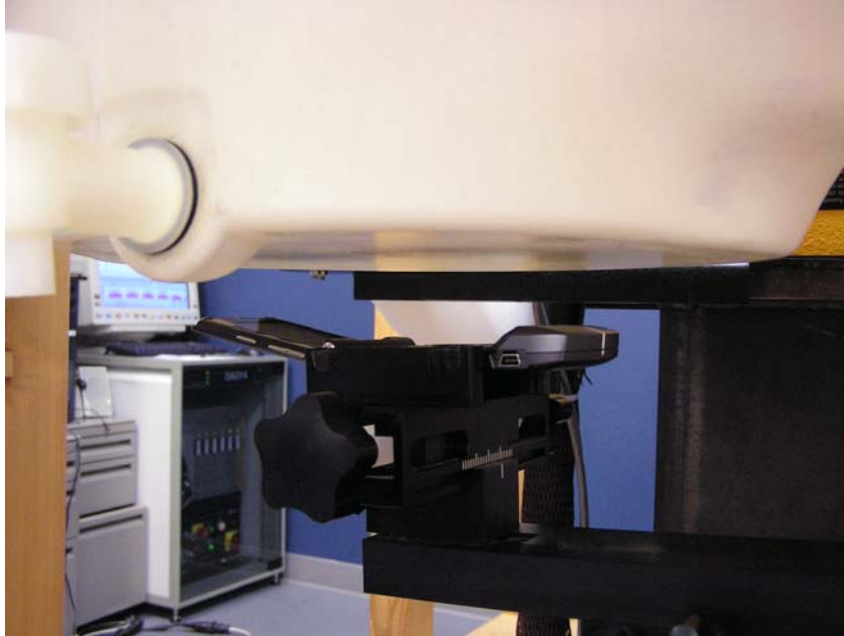
Figure 9 – Transceiver in Face Dispatch position, 25 mm from Phantom
