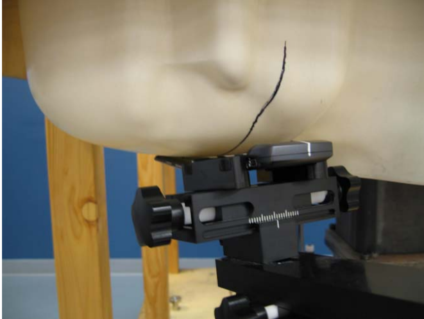
Figure 5 – Transceiver against head, Cheek Touch position
