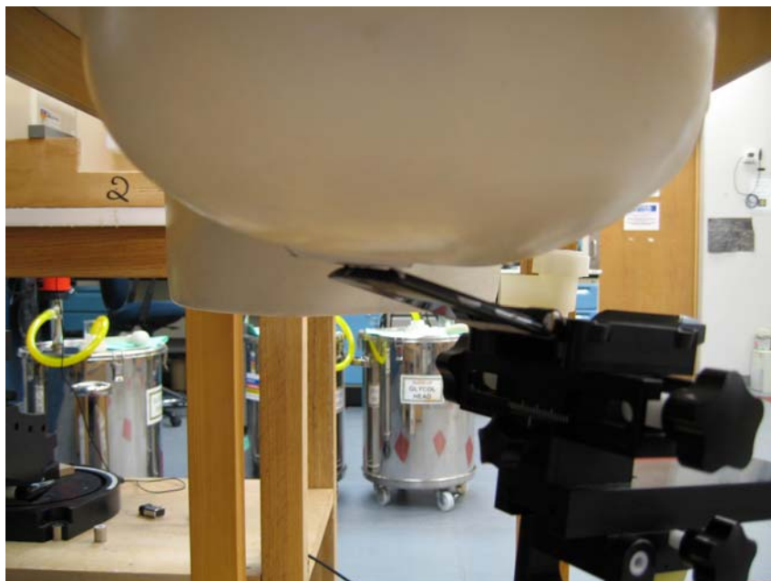
Figure 8 – Transceiver against head, 15° Tilt position
