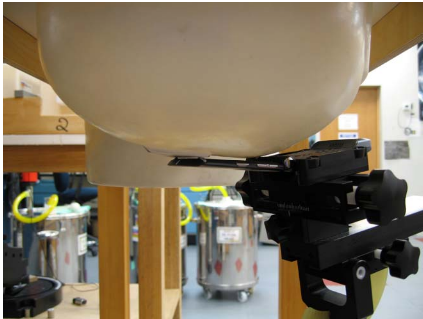
Figure 6 – Transceiver against head, Cheek Touch position
