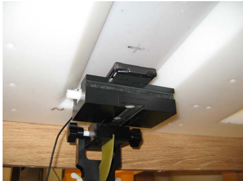
Figure 10 – Transceiver against body, Back of Phone 15 mm from Phantom position
