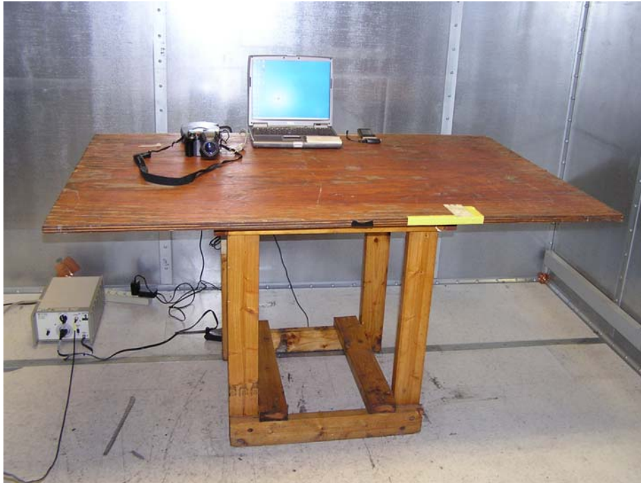
Figure 1. AC Line Conducted Emissions Measurement Setup
