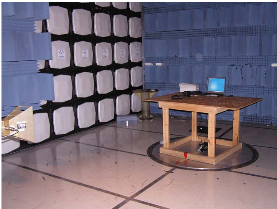
Figure 2. Part 15 Radiated Emissions Measurement Setup
