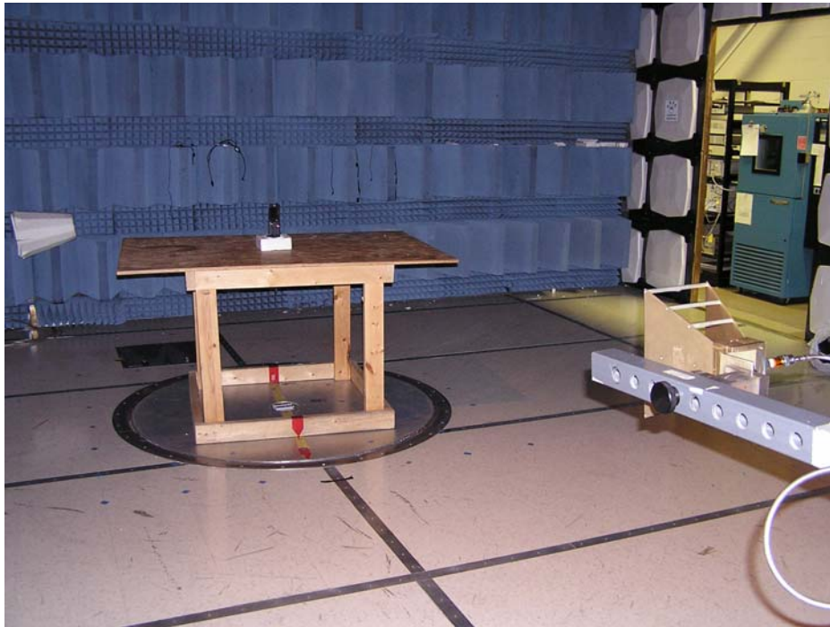
Figure 3. Part 22/24 Radiated Emissions Measurement Setup
