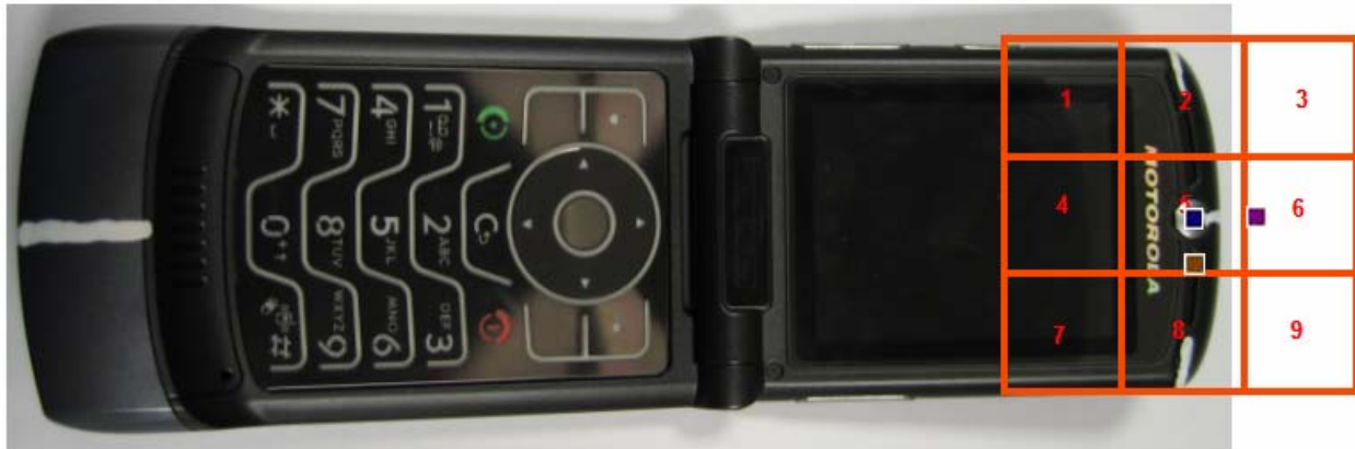
Figure A4-3. Phone Open – Location of Measured Points for T-coil – 5cm x 5cm grid for Near Field Measurements
