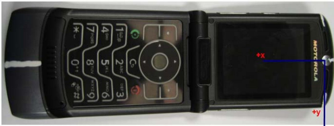
Figure A4-2. Phone Open – Coordinate Axis for T-coil Measurements
