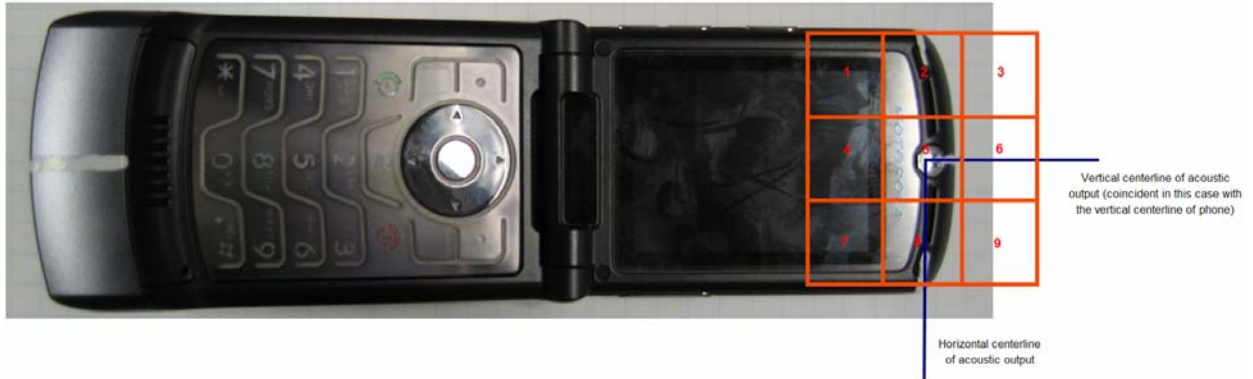
Figure A6-1. Phone Open - Orientation of Wireless Device and Measurement Plane
