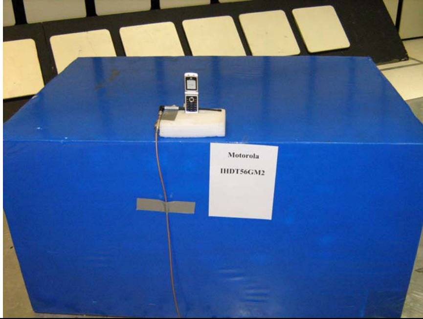
Figure 1 Test setup for Radiated Emissions
