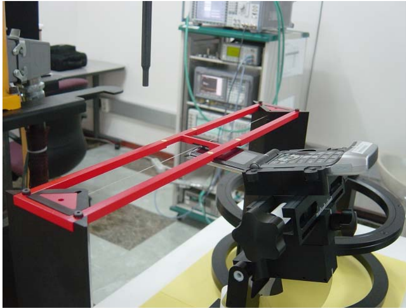
Figure A5-4. Positioning for RF Emissions
