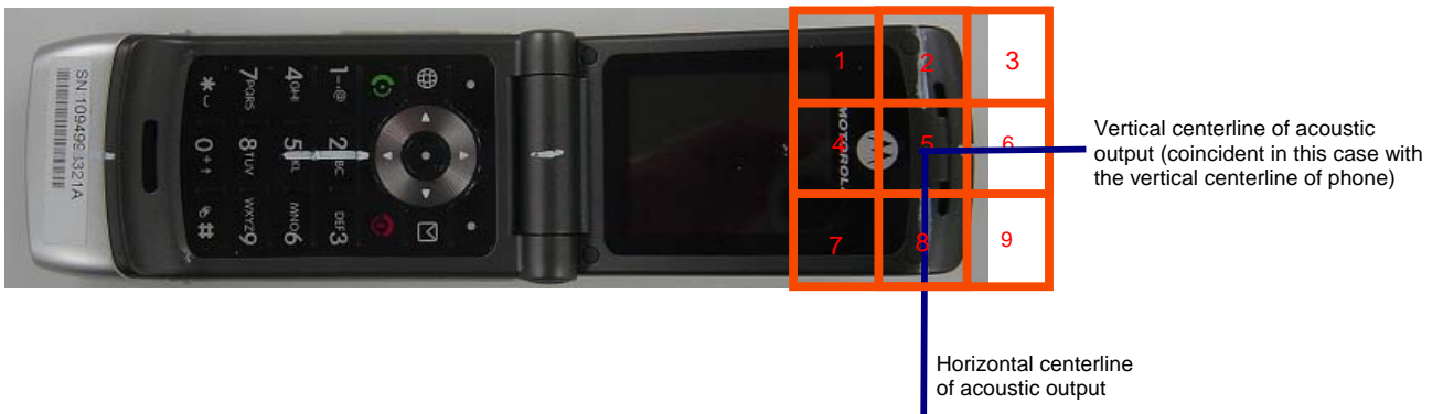
Figure A5-3. Phone Open - Orientation and Measurement Plane for RF Emissions Testing
