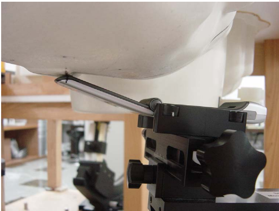
Figure 6. Phone Against the Head Phantom (15°Tilt)
