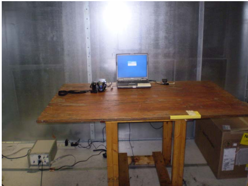
Figure 2. Computer Peripheral AC Line Conducted Emissions Measurement Setup
