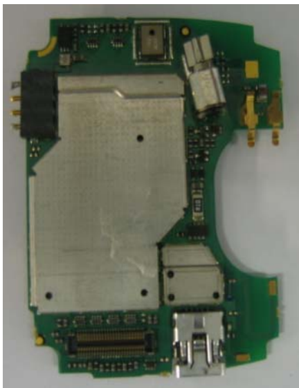
Main board top with shields
