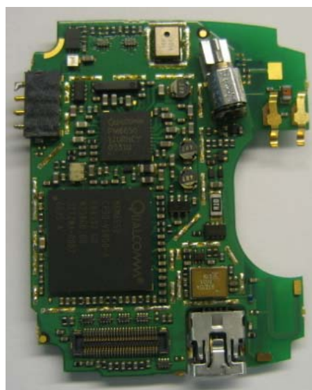
Main board top without shields
