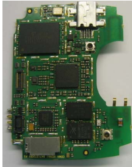
Main board bottom without shields
