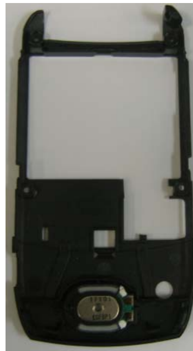
Inside front transceiver housing
