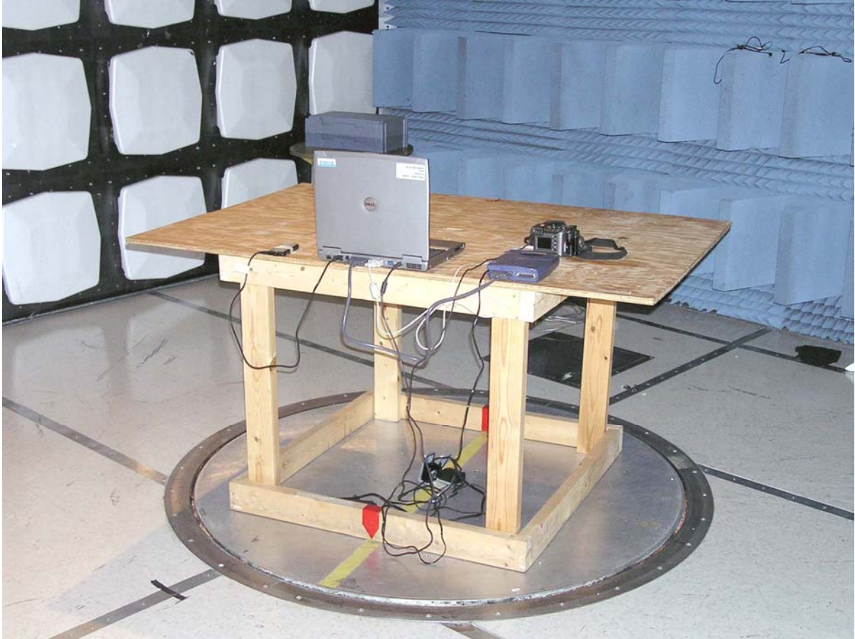
Radiated Emissions Measurement Setup (Representative Photo- Not Actual Phone Tested)
