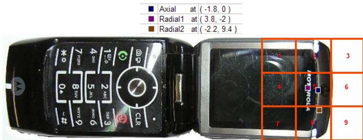
Figure A4-3. Phone Open – 5cm x 5cm grid for Near Field Measurements and T-coil Measured Point locations
