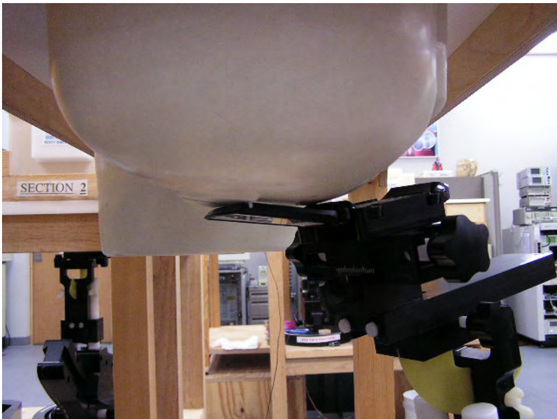
Figure 5 – Transceiver against head, Cheek Touch position
