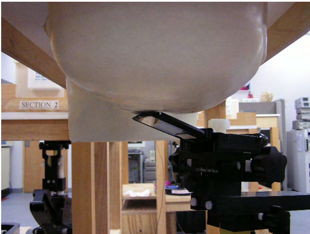
Figure 7 – Transceiver against head, 15° Tilt position
