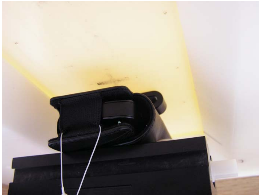
Figure 4 – Bodyworn Against Flat Phantom
