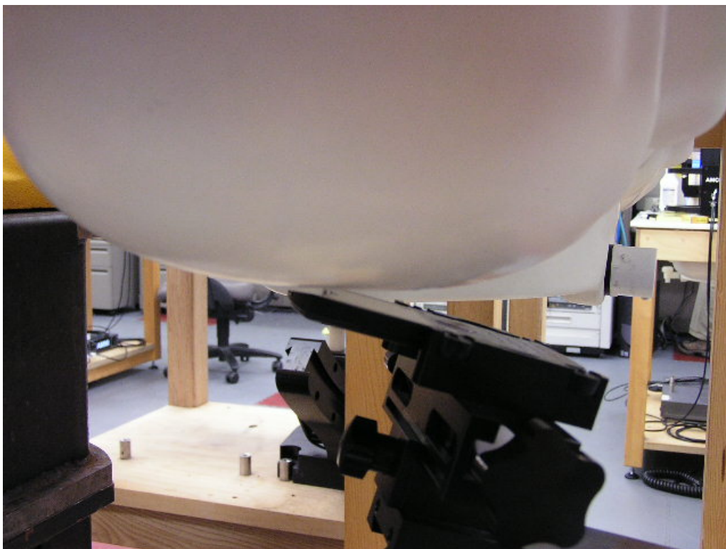
Figure 3 – Transceiver against head, 15° Tilt position
