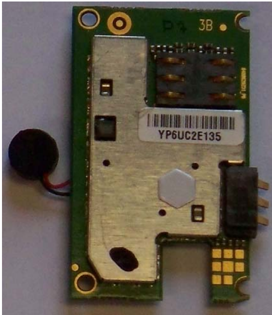
Main Board Top With Shields
