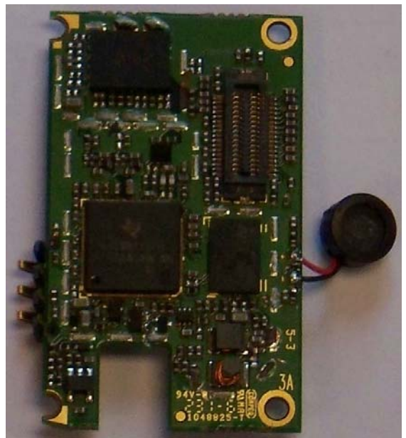
Main Board Bottom Without Shields
