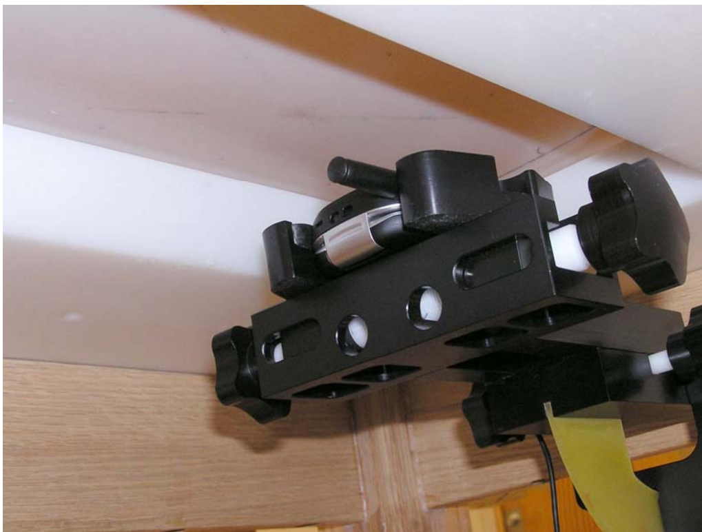
Figure 11. Phone Against the Flat Phantom with antenna retracted
