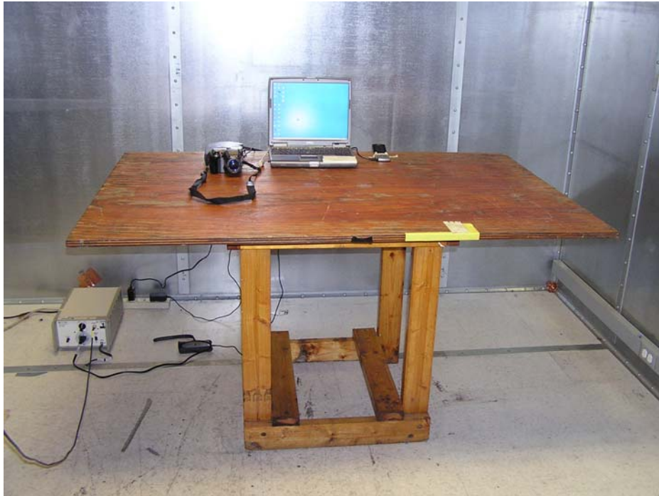
Figure 1. AC Line Conducted Emissions Measurement Setup
