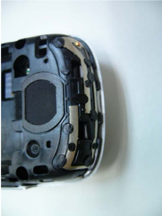
Top view of GSM antenna
