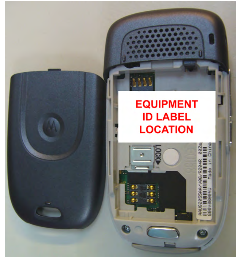
Rear View with Battery Cover Removed Showing ID Label
