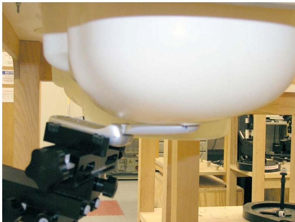
Figure 4. Phone Against the Head Phantom (Cheek Touch)
