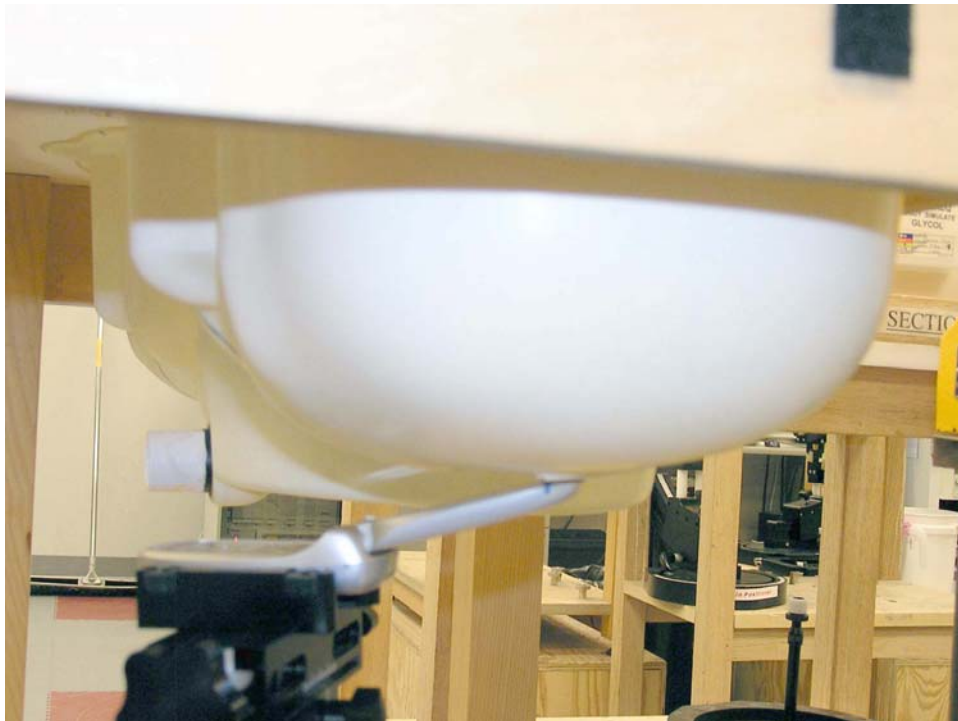
Figure 5. Phone Against the Head Phantom (15° Tilt)
