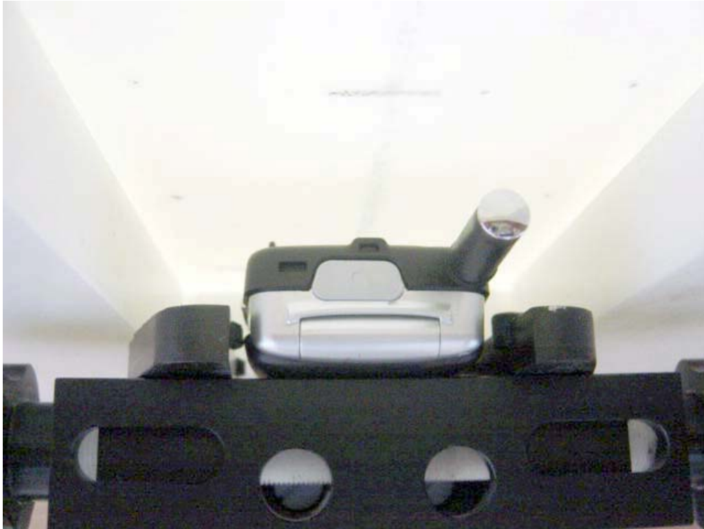
Figure 7. Phone Against the Flat Phantom; antenna retracted
