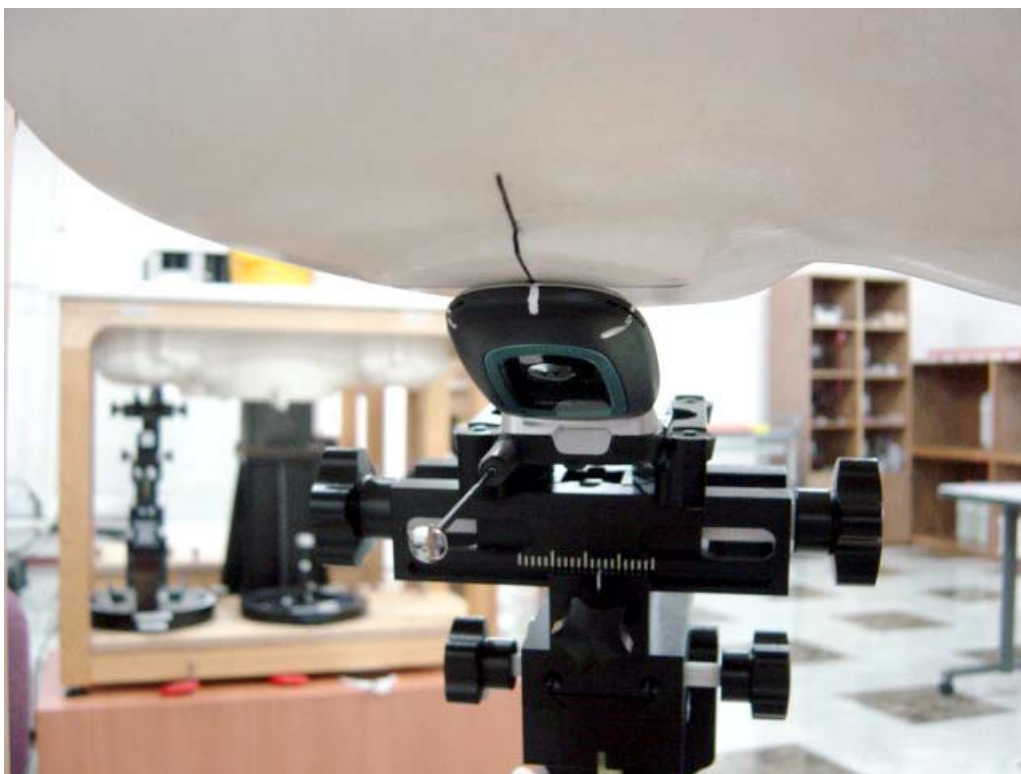
Figure 14. Phone Against the Head Phantom (rear view, 15°Tilt, antenna extended)
