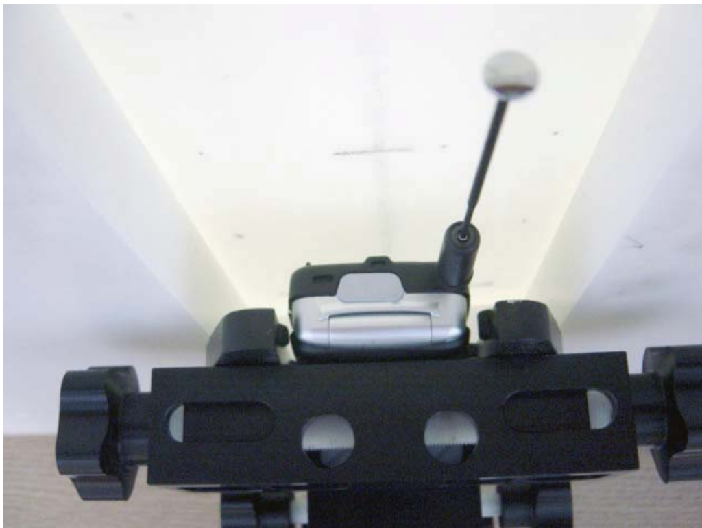
Figure 8. Phone Against the Flat Phantom; antenna retracted
