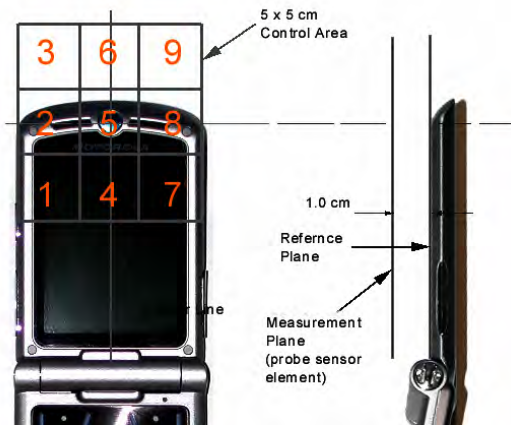
Figure 13 E/H-Field Emissions Test Setup Diagram
