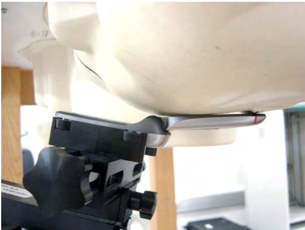
Figure 5. Phone Against the Head Phantom (Cheek Touch)
