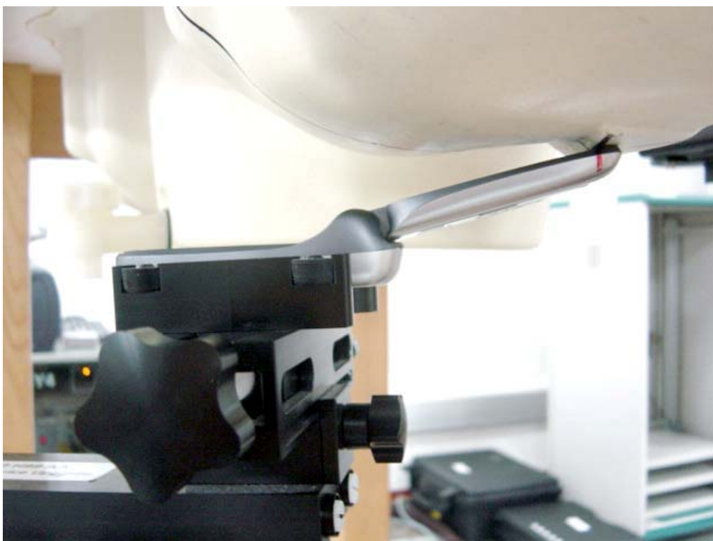
Figure 6. Phone Against the Head Phantom (15°Tilt)
