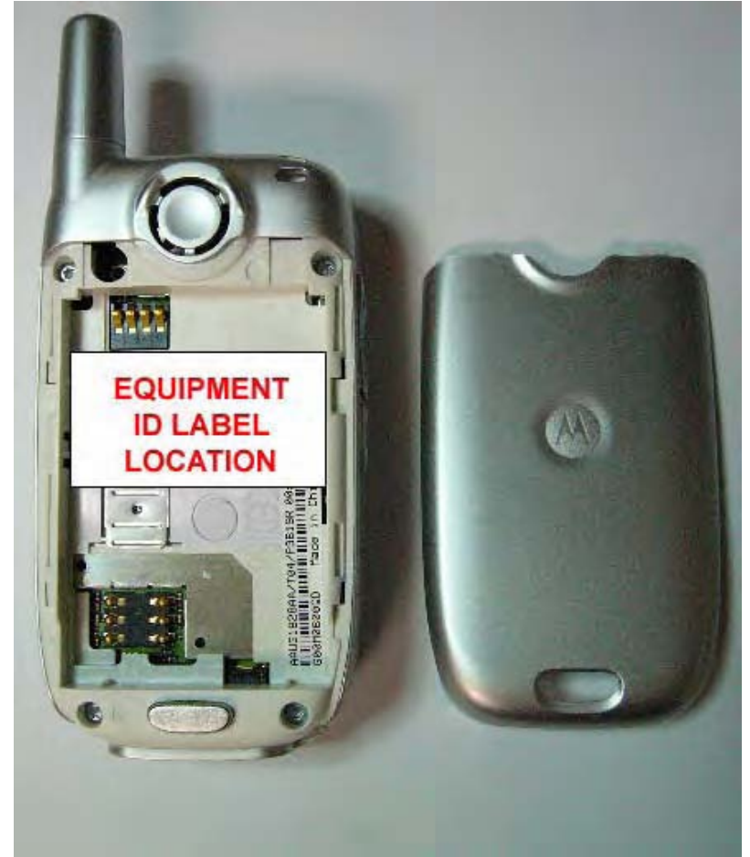
Rear View with Battery Cover Removed Showing ID Label
