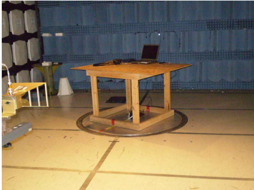
Figure 2. Computer Peripheral Radiated Emissions Measurement Setup
