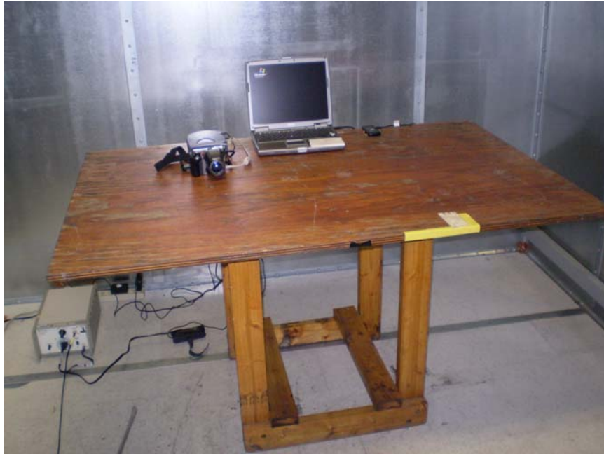
Figure 1. Computer Peripheral AC Line Conducted Emissions Measurement Setup
