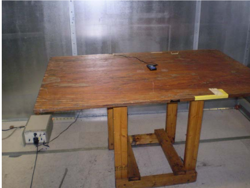
Figure 3. AC Line Conducted Emissions Measurement Setup
