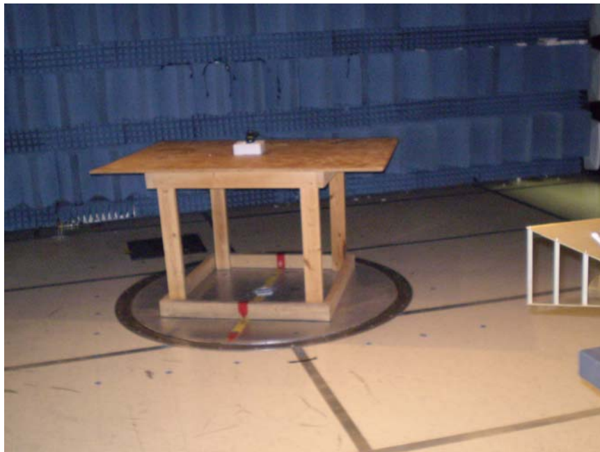
Figure 4. Radiated Emissions Measurement Setup
