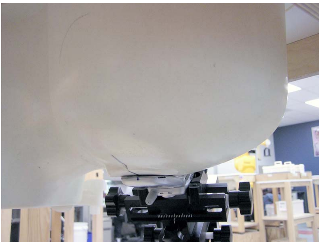
Figure 6. Phone Against the Head Phantom (Back View - Cheek Touch)
