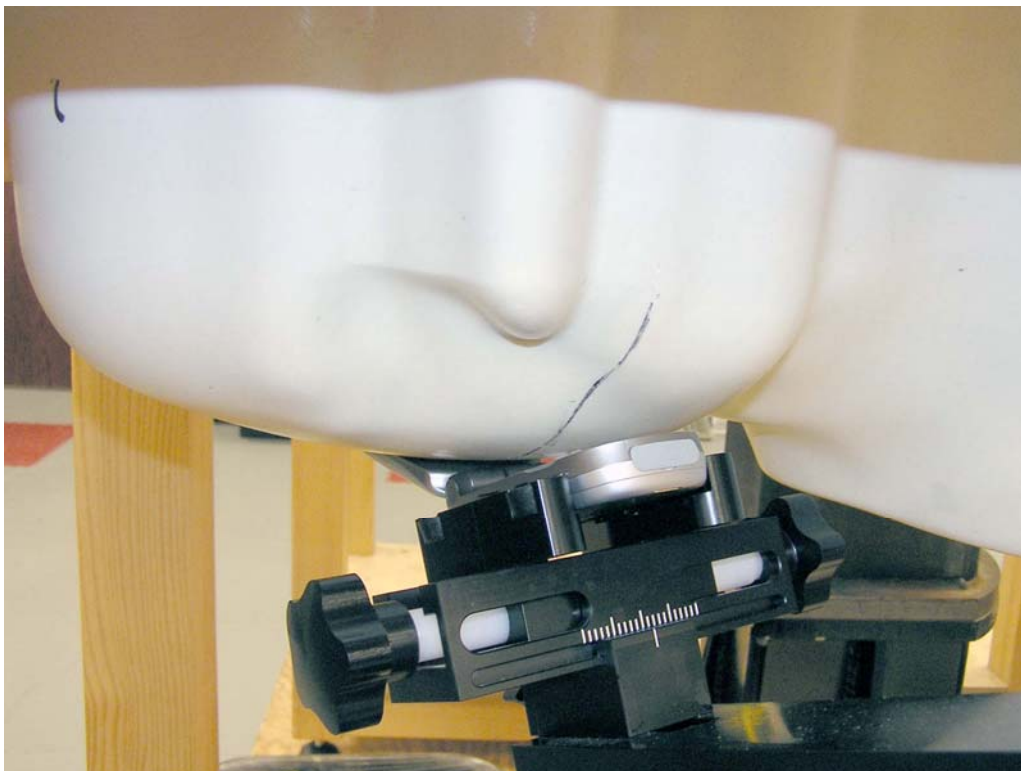
Figure 5. Phone Against the Head Phantom (Front View - Cheek Touch)
