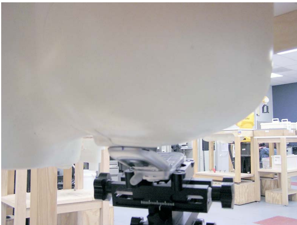
Figure 8. Phone Against the Head Phantom (Back View – 15°Tilt)
