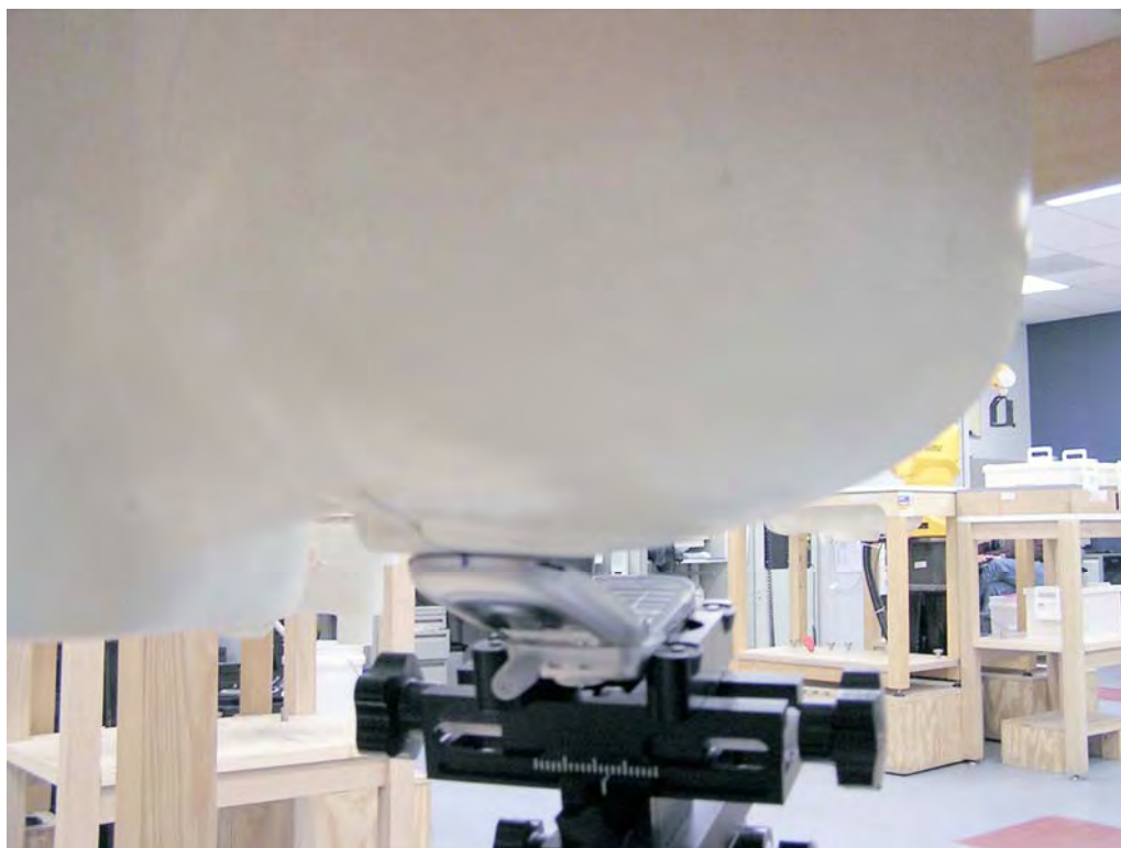
Figure 8. Phone Against the Head Phantom (Back View – 15°Tilt)
