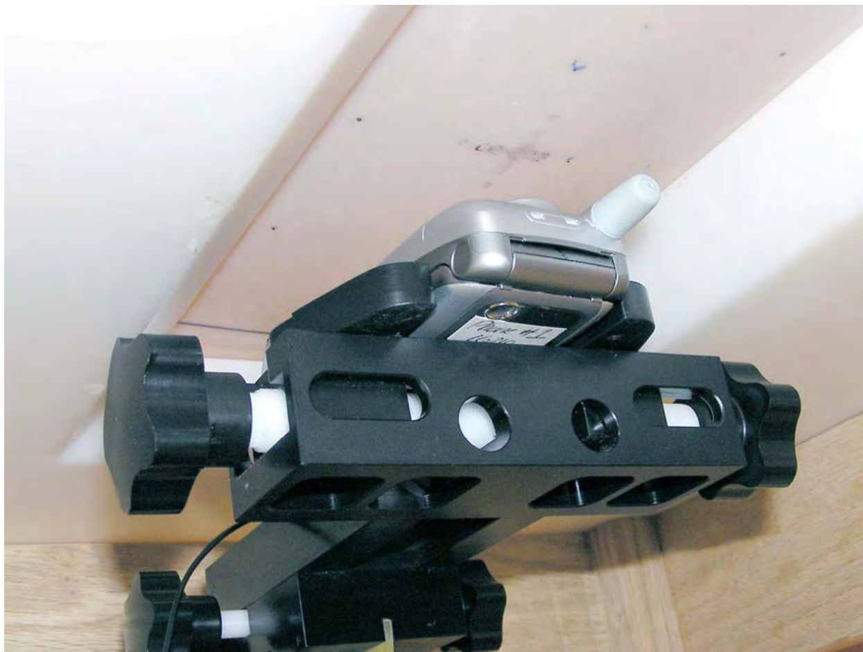
Figure 4. Phone Against the Flat Phantom
