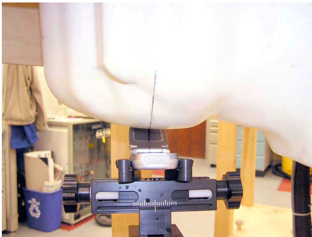
Figure 7. Phone Against the Head Phantom (Front View – 15°Tilt)
