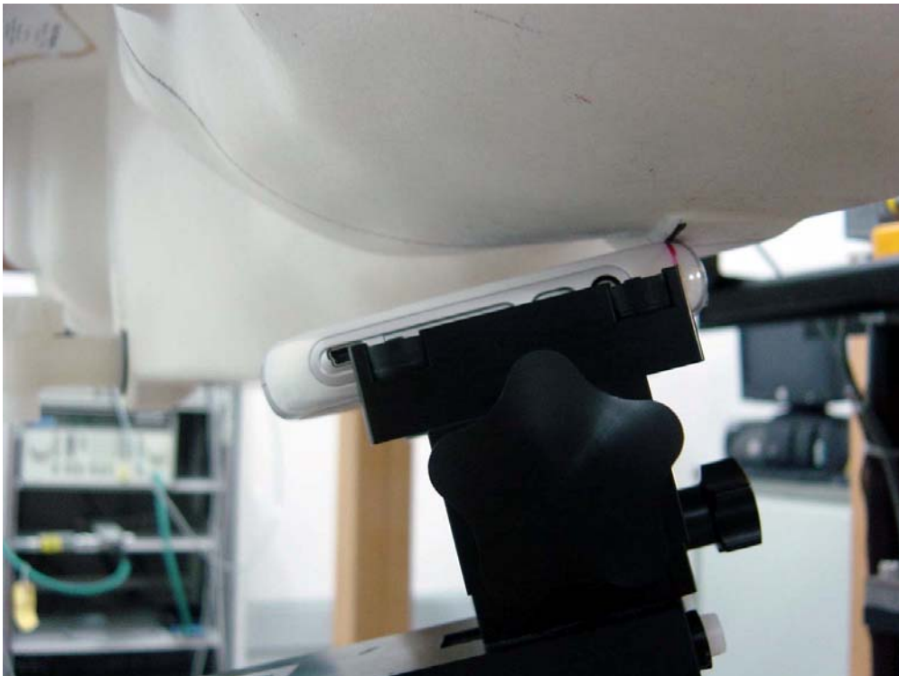
Figure 4. Phone Against the Head Phantom (15°Tilt)
