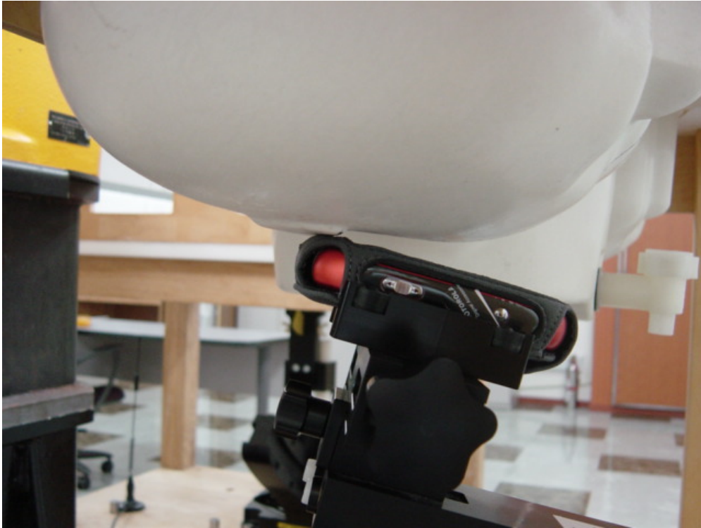
Figure 11. Phone with Arm Band Case SYN1697A Against the Head Phantom (15°Tilt)
