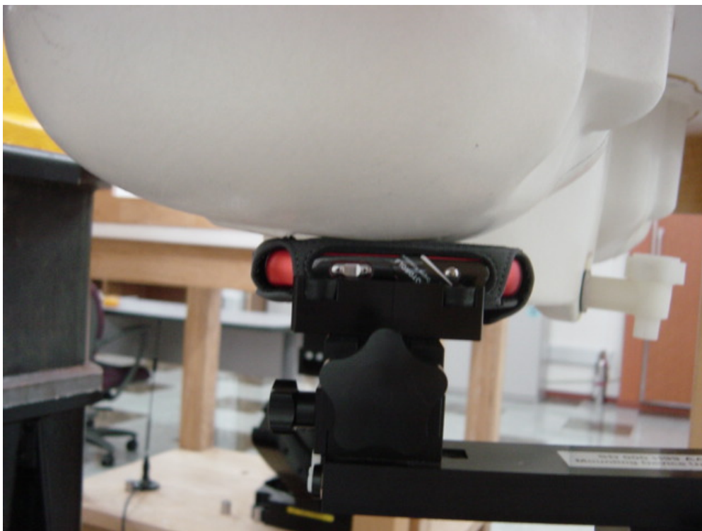
Figure 10. Phone with Arm Band Case SYN1697A Against the Head Phantom (Cheek Touch)
